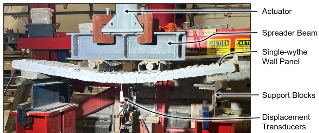
Figure 3: Experimental test setup and instrumentation
