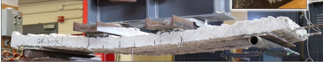
Figure 6: Deflected shape at the ultimate load and failure modes for 3D printed wall panels with NSM reinforcement: (a) GFRP-reinforced panel (W4-GFRP-E), (b) steel-reinforced panel (W2-Steel-E).
